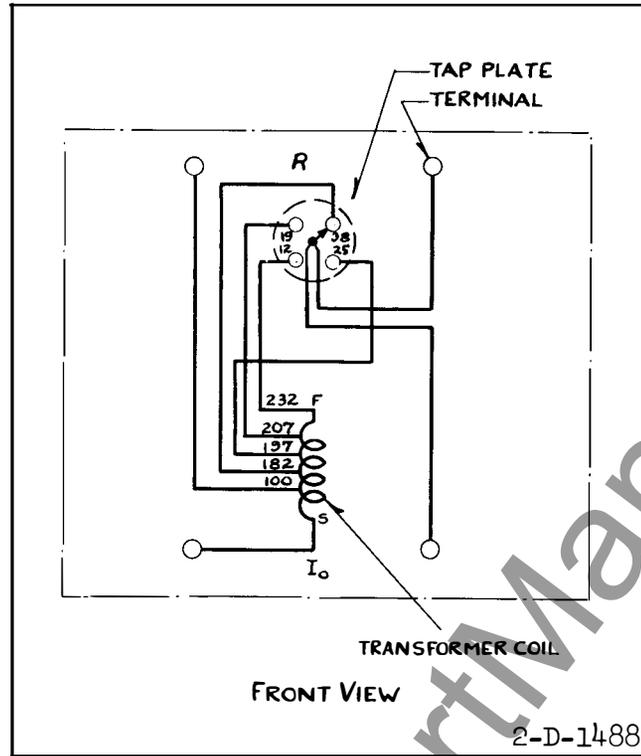
Fig. 12. Internal Schematic for the Auxiliary Current Transformer.
