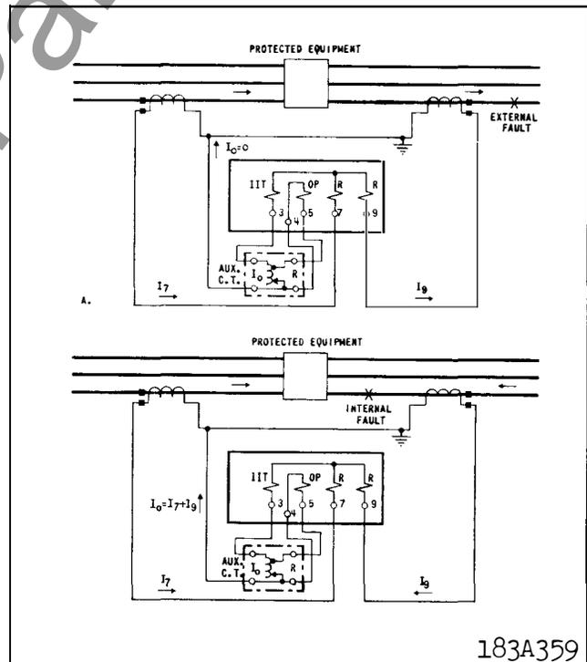
\* Fig. 3. Schematic Diagrams of the Type CA-5 Relay. (A) Shows the Fault Current Distribution for an External Fault; (B) The Distribution for an Internal Fault.
