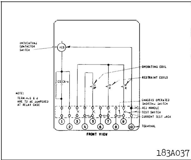
Fig. 1. Internal Schematic of the Type CA-5 Relay in the Type FT21 case.
