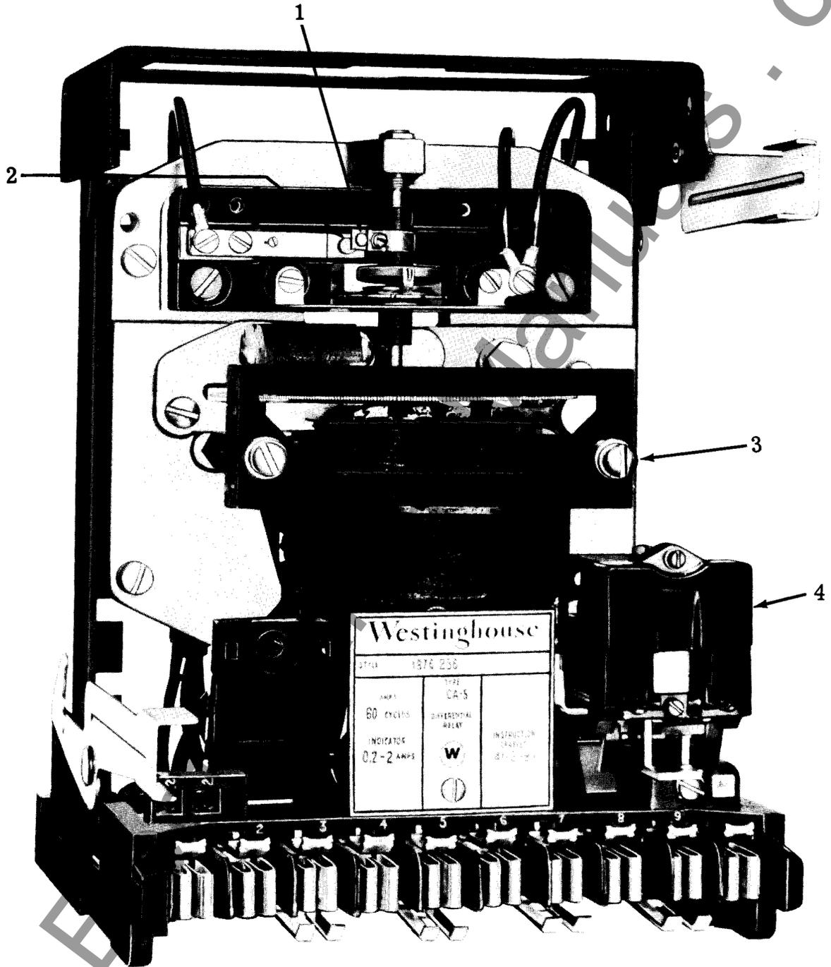
Fig. 14. Types CA-5 Relay Without Case (Front View). 1—Moving Contact. 2—Stationary Contact. 3—Two Electromagnets (front restraint electromagnet with two windings; rear operating electromagnets with single winding). 4—Indicating Contactor Switch (ICS).
