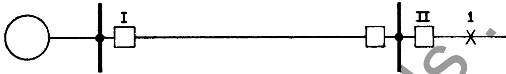
FIG. 1 OPERATION OF PROTECTED RELAY, I, SHOULD BE DELAYED TO PERMIT THE PROTECTING RELAY, II, TO CLEAR FAULT 1.
