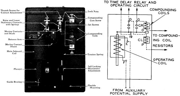
FIG. 1—RELAY WITH COVER REMOVED
