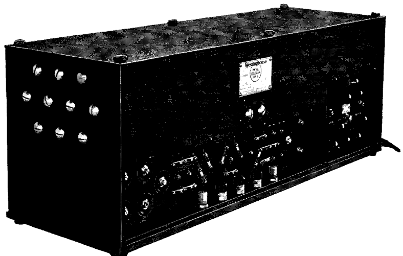
FIG. 3—REAR VIEW OF MAIN UNIT SHOWING LAMP TERMINALS AND CURRENT TERMINALS
