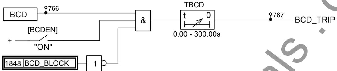
**Figure 2.4.10.3 Broken Conductor Protection Scheme Logic**
