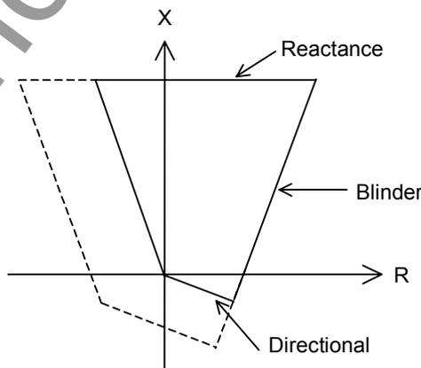
**Figure 2.6.1.11 Quadrilateral characteristic**
