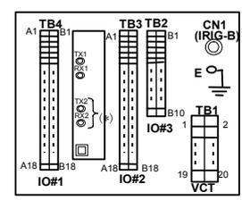
**Terminal Block Arrangement (Rear view)**
