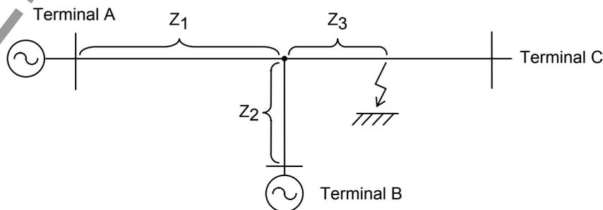
Figure 2.3.2.1 Three-terminal line
