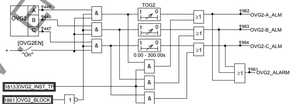
Figure 2.4.9.5 OVG2 Overvoltage Protection
