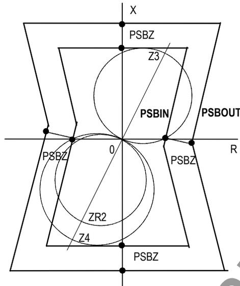
Figure 2.6.1.4 Power Swing Blocking Element
