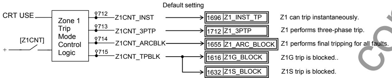
Figure 2.4.1.7 Zone 1 Trip Mode Control Circuit
