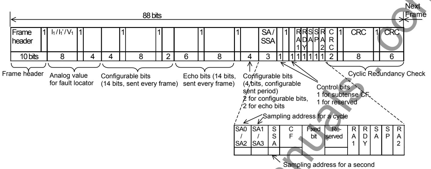
$I_1 / I_1' / V_1$ : 12 bits sent every three frames
