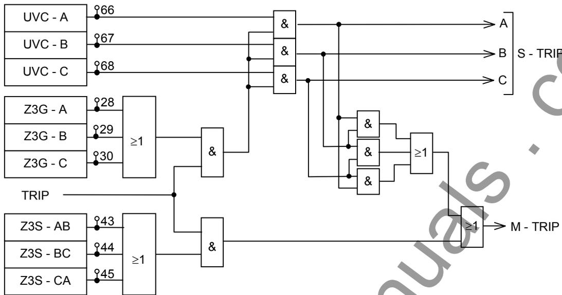
Figure 2.4.3.9 Phase Selection Logic for Command Protection
