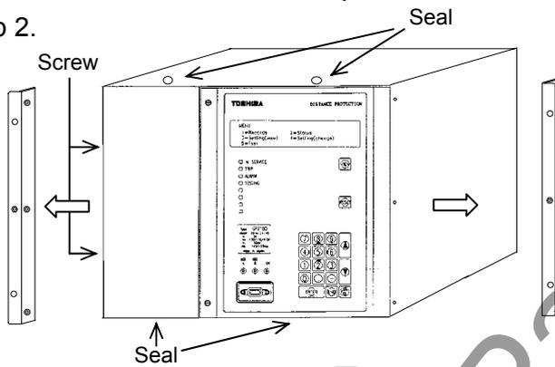
Remove the left and right brackets by unscrewing the three screws respectively, then remove two screws on left side of the relay.
