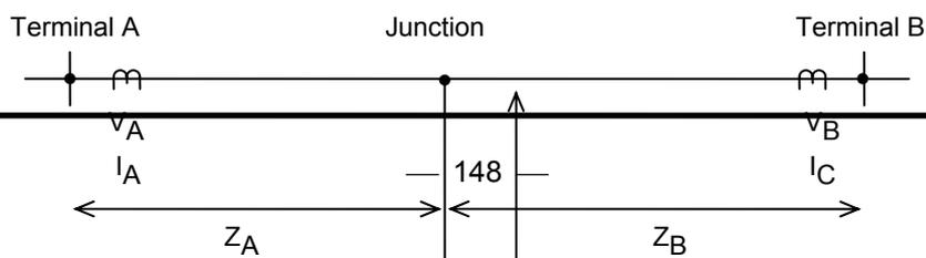
Figure 2.8.4.2 Three-terminal Model
