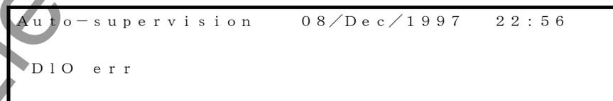
If the automatic supervision function detects a failure while the LCD is off, the "Auto-supervision" screen is displayed automatically, showing the location of the failure and the "ALARM" LED lights.
