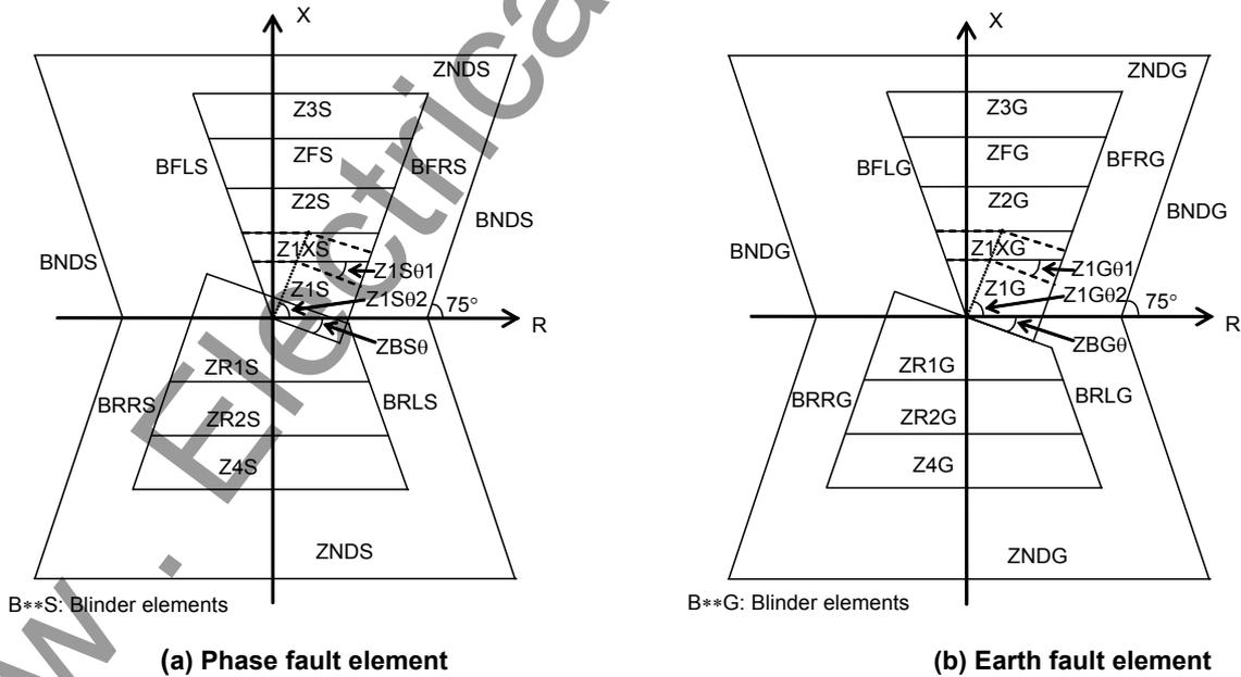
Figure 2.4.1.2 Quadrilateral Characteristics
