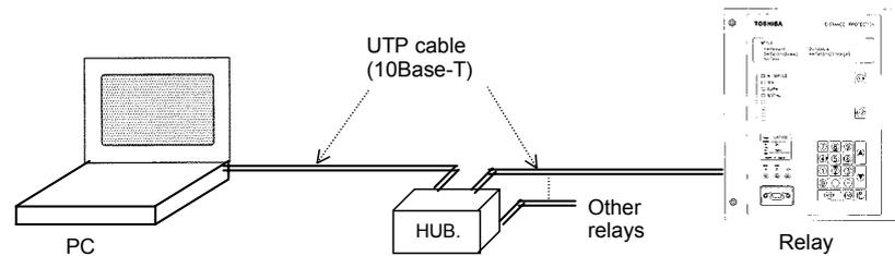
Figure 4.4.2 Relay Setting and Monitoring System (2)
