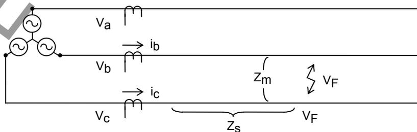
Figure 2.2.1.1 Two-Phase Fault
