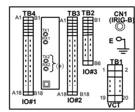
**Terminal Block Arrangement (Rear view)**
