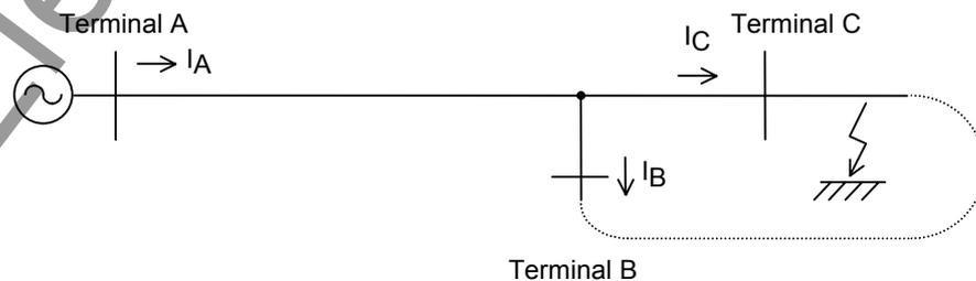
**Figure 2.3.2.3 Outfeed Current in Event of External Fault**
