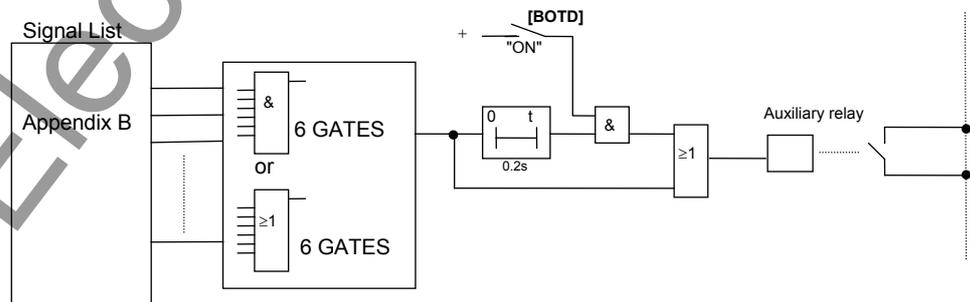
Figure 3.2.2.1 Configurable Output
