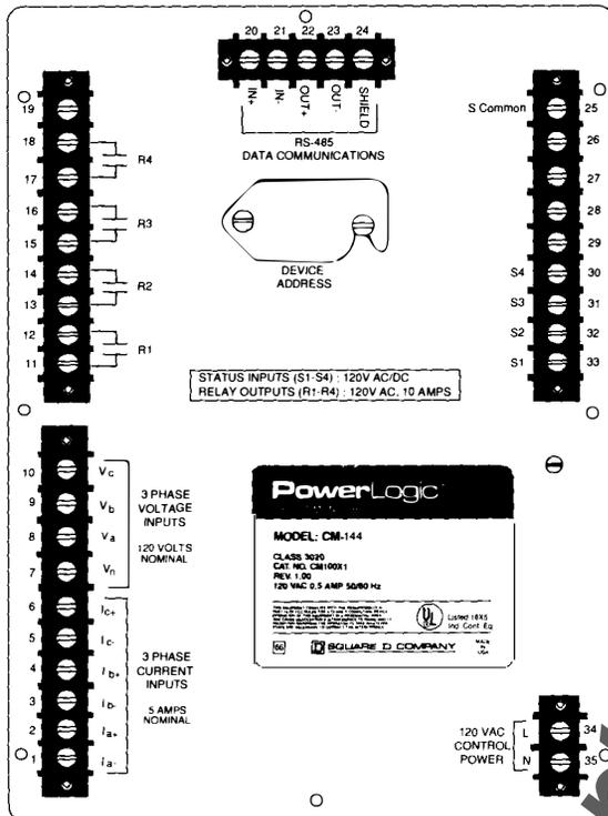
**Circuit Monitor with 4 Status Inputs, 4 Relay Outputs**
