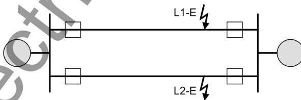
Figure 2-2 Multiple fault on a double-circuit line
