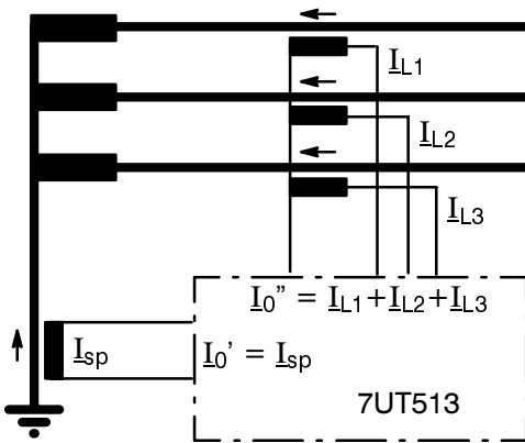
Figure 4.27 Principle of restricted earth fault protection
