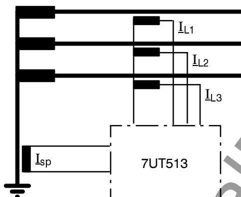
Figure 4.24 Restricted earth fault protection on an earthed transformer winding
