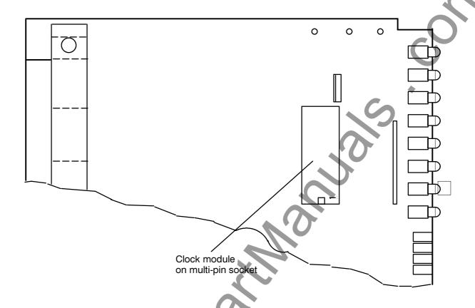
Figure 7.1 Position of the clock module
