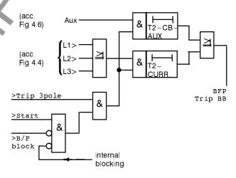
Figure 4.9 Breaker failure protection with common phase initiation
