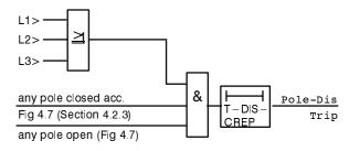
Figure 4.19 Function scheme of pole discrepancy supervision
