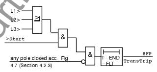
Figure 4.18 Function scheme of end fault protection
