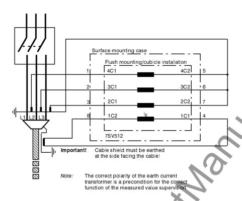
Figure B.4 Connections to three current transformers – residual current fed from particular summation c.t., preferably for effectively earthed or low-ohmic earthed systems
