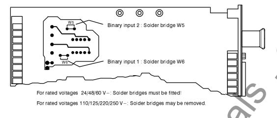
Figure 5.1 Checking of control voltages for binary inputs 1 and 2
