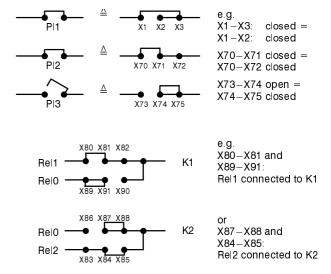
Figure 5.5 Plug jumper arrangement
