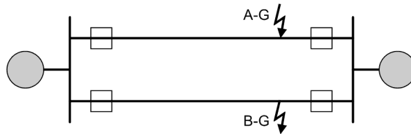
Figure 2-5 Multiple fault on a double-circuit line
