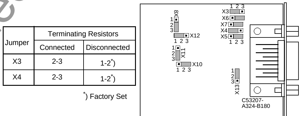
Figure 8-8 Location of the Jumpers for Configuring the Terminating Resistors of the Interface on Card Version C53207-A324-B180
