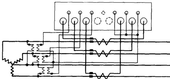
21. WD 3-Phase 4-Wire 3-Element Wye with Current and Potential Transformers
