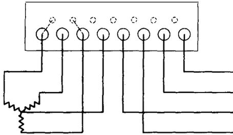
16. WDP and WD 3-Phase 4-Wire 2-Element Wye Self Contained
