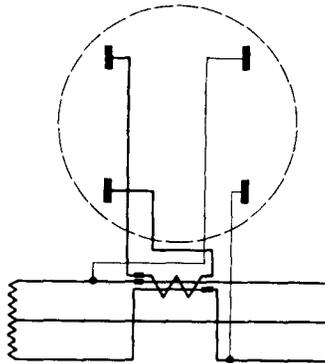
25. WDS Singlephase 2-Wire Meter Used on 3-Wire Circuit with 3-Wire Current Transformer
