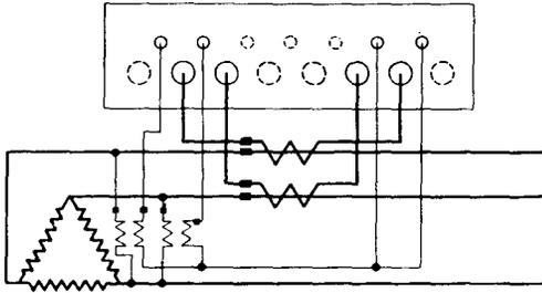
15. WDP and WD 3-Phase 3-Wire with Current and Potential Transformers
