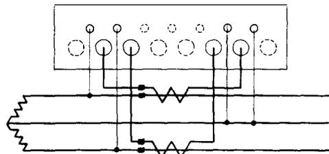
13. WDP and WD 3-Phase 3-Wire with Current Transformers on Network Service
