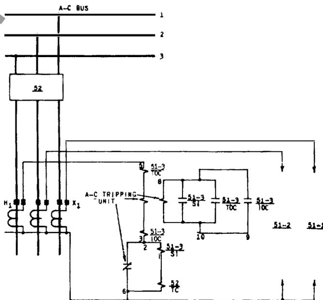
Fig. 6 (K-6375669-6) External Connections of Three Type IAC51R Relays used for 3-Phase Circuit Protection.
