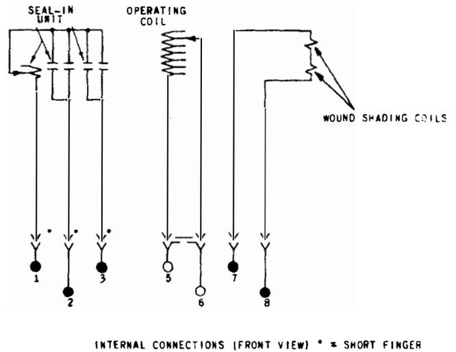
Fig. 6 (K-6400203-4) Internal Connections For Type IAC61A Relay (Front View)
