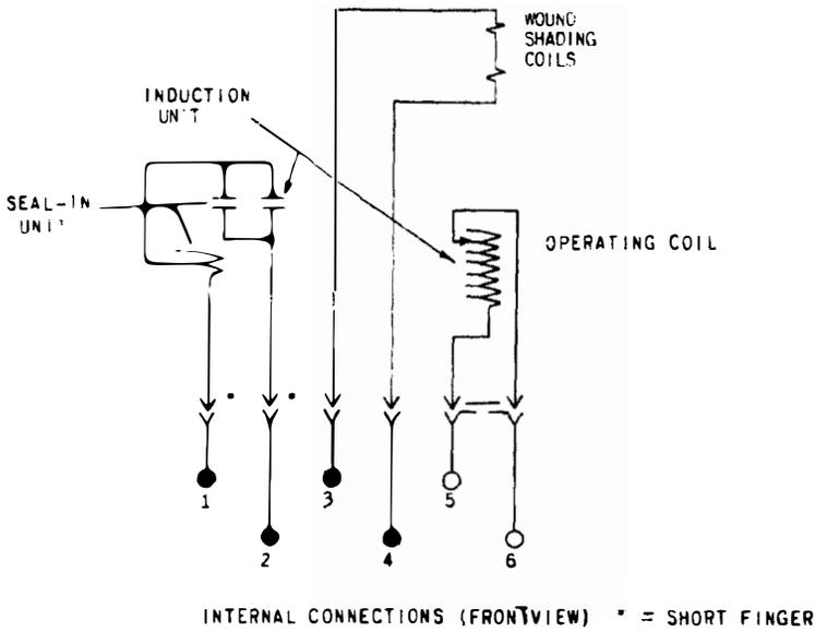
Fig. 3 (K-6306994-4) Internal Connections For Type IAC60A Relay (Front View)
