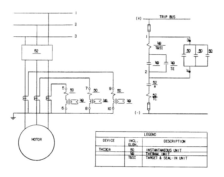
Figure 2. (0246A3683-0) Typical External Connections for Type THC30A Relay
