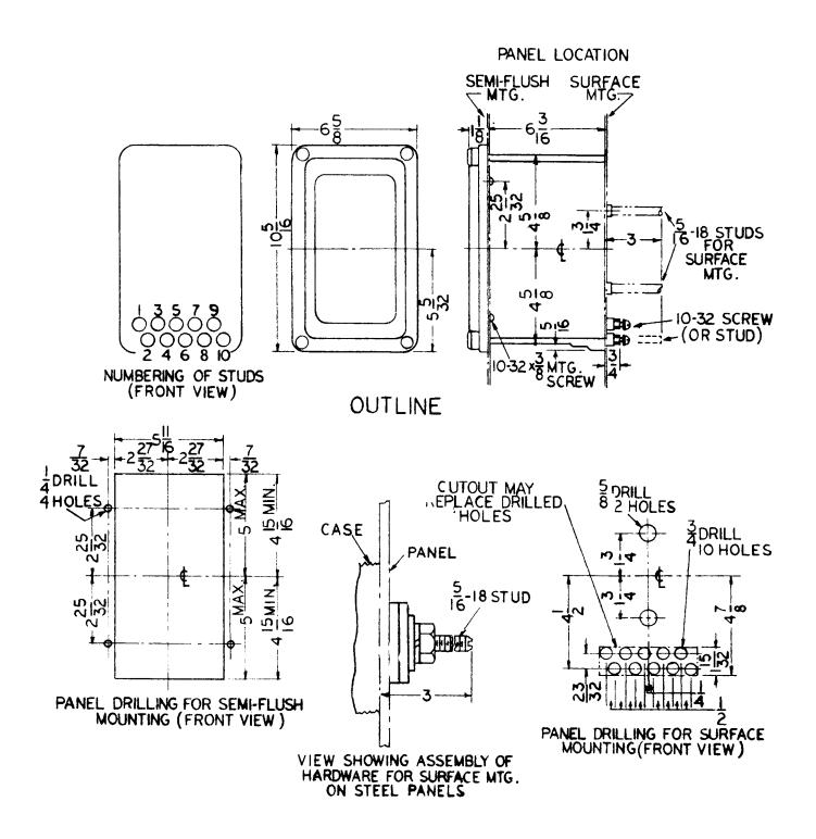
Figure 4. (0227A8541-0) Outline and Panel Drilling for THC30A Relay
