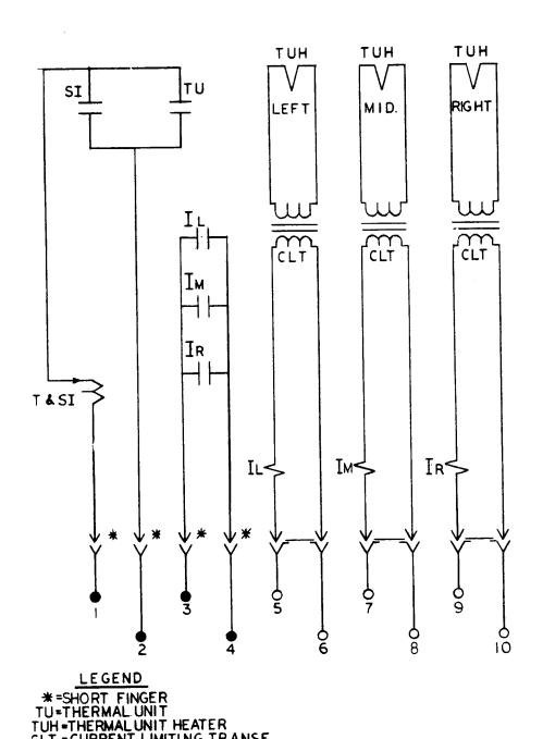
CLT = CURRENT LIMITING TRANSF. T&SI = TARGET & SEAL-IN IL.IM. IR = INSTANTANEOUS UNIT (LEFT, MIDDLE, RIGHT)
