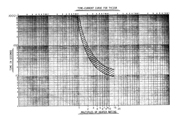
Figure 3. (0246A3824-0) Time Current Curve for THC30A
