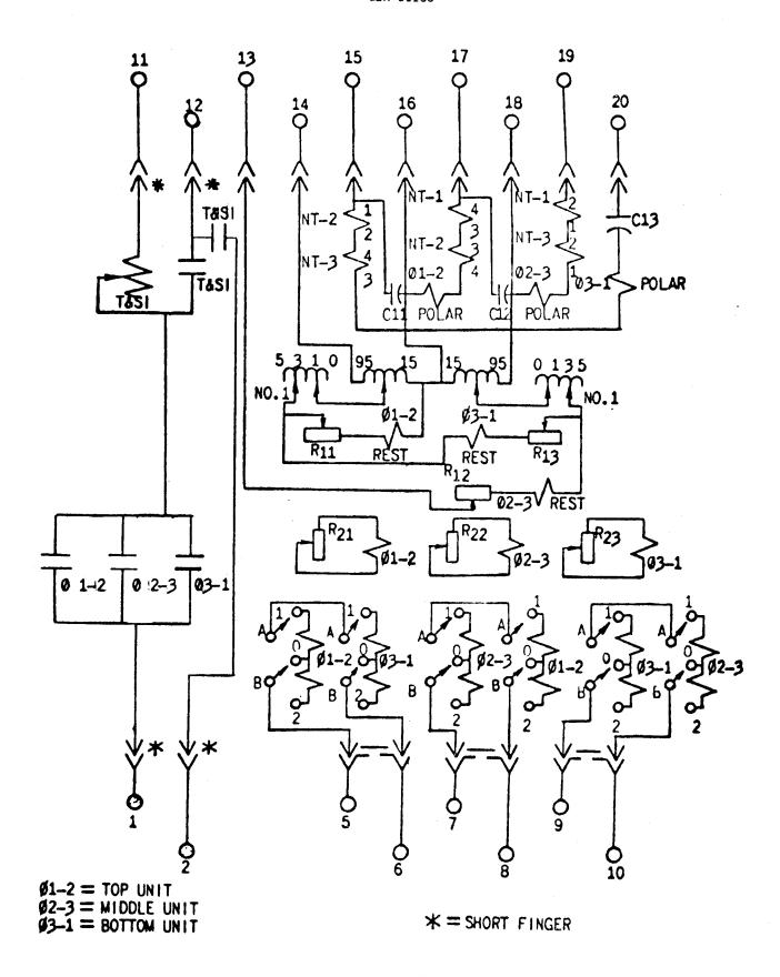
FIG. I (0208A2464-0) Internal Connections Diagram For The CEY54A Relay (Front View)
