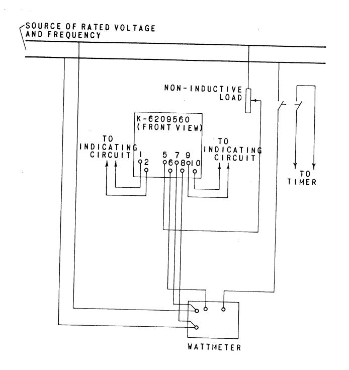
Fig. 4 (K6209602 [2]) Testing Connections for Type CFW11E Relay Using Wattmeter
