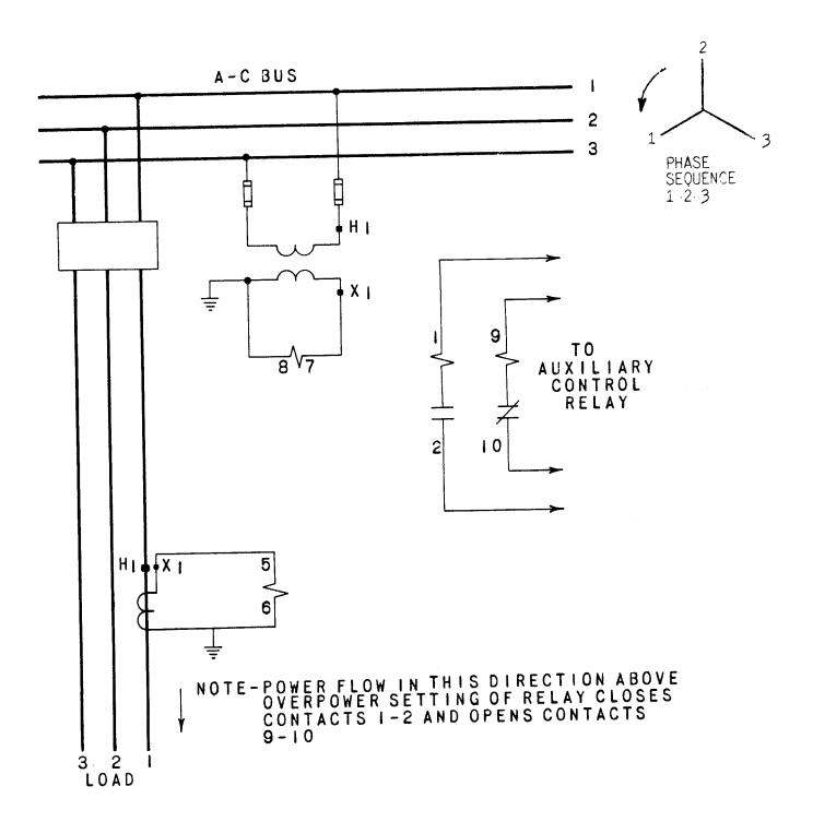
Fig. 3 (K-6209604-2) Typical External Connections for Type CFW11E Relay
