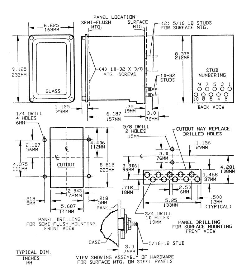
Fig. 7 (6209271 [8]) Outline and Panel Drilling for Type CFW11E Relay
