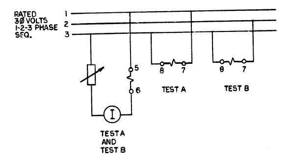
Fig. 5 (0275A3258-0) Testing Connections for Type CFW11E Relay Using Three Phase Voltage Source
