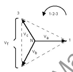
$V_f$  = Desired Fault Voltage
