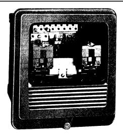
Hi-Lo CO induction-disc type overcurrent relays are activated when the current in them exceeds given values. The circuit closing type relays are normally used to trip a circuit breaker. They may have either single or double contacts for tripping one or two circuit breakers.
