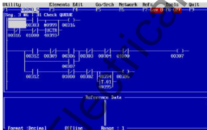
Figure 35 – Segment 3 Network 6- XMIT Dwell Timer And Bad Transmission Counter Logic.
