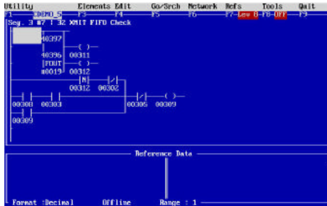
Figure 36 – Segment 3 Network 7 – FIFO Empty/Full Notification Logic
