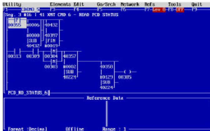
Figure 45 – Segment 3 Network 16 – Read PCD Status Information Or FIFO Instruction Load.
