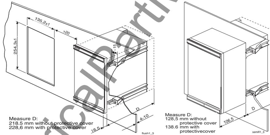
Fig. 5 Flush mounting and semi-flush mounting of REA 101
