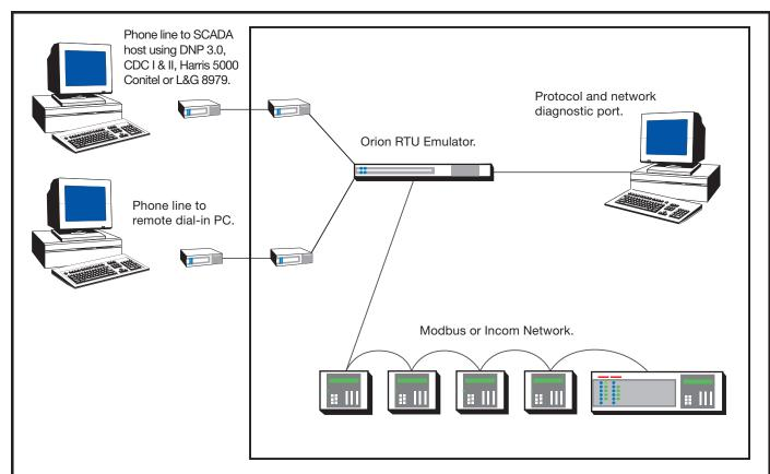
Figure 1. Typical Orion installation in substation showing connections on all four serial ports: to ABB Relays, to SCADA host computer, to dail-in computer and to local diagnostic computer.
