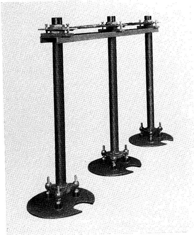
FIG. 11. Moving Electrode Assembly Showing Bolts for Adjusting Electrode Position
