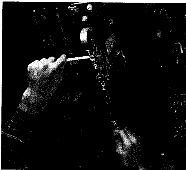
FIGURE 34—Measuring Contact Spring Pressure
