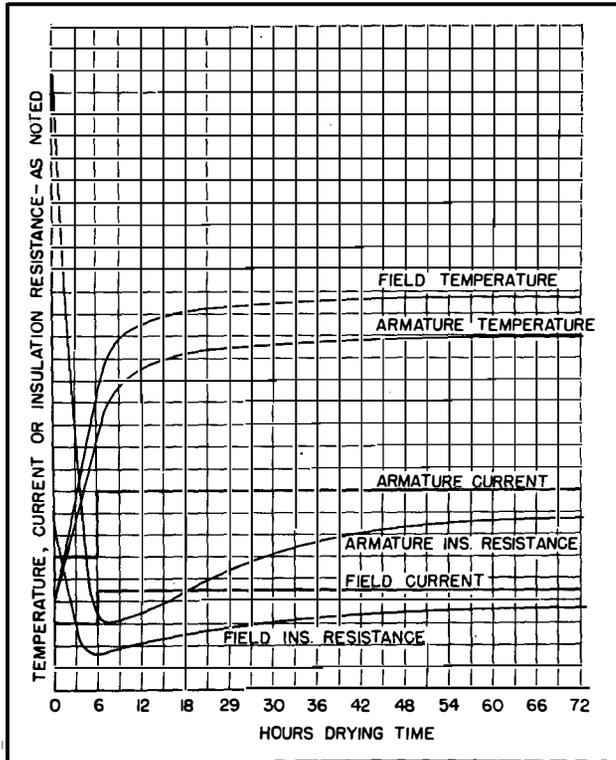
FIG. 23. Typical Insulation Resistance Curve
