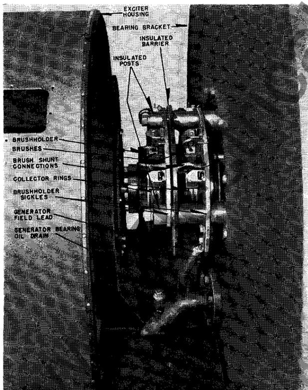
FIG. 9. Exciter Housing Rolled Back Giving Access to Collector
