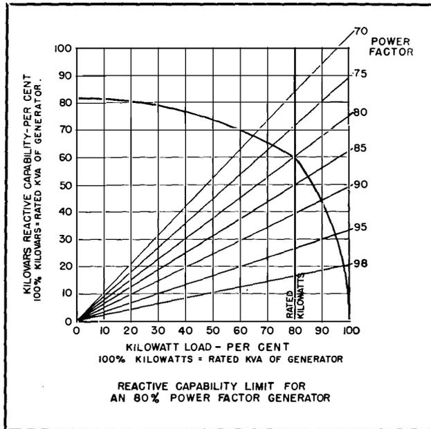
FIG. 24. Reactive Capability Curve
