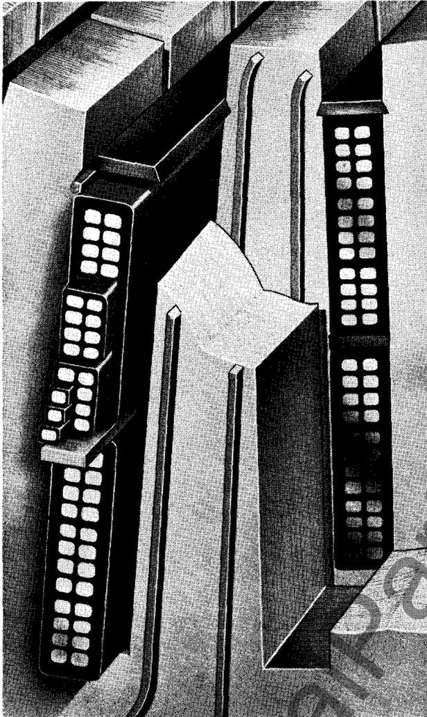
FIG. 2. Stator Coil Insulation
