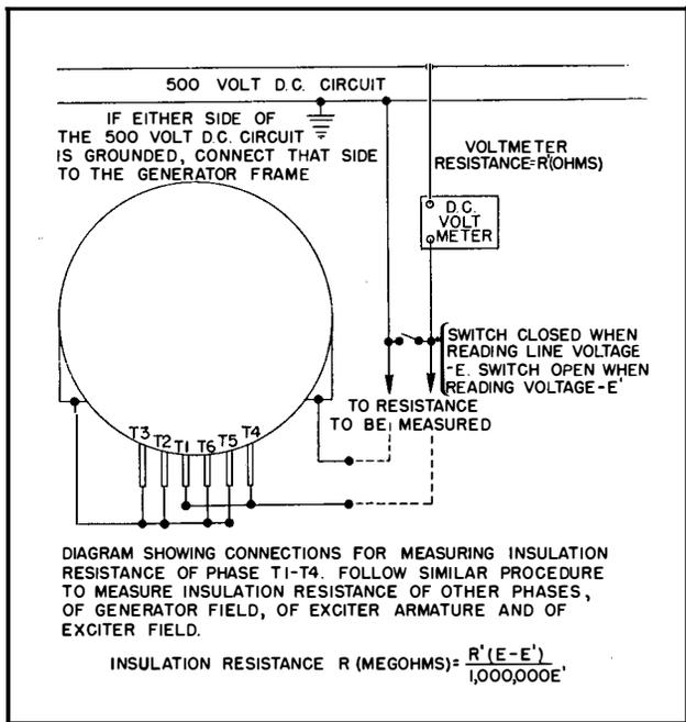
FIG. 21. Connections for Insulation Resistance Measurement
