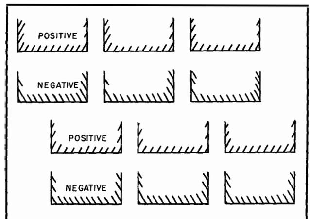
FIG. 27. Correct Method of Staggering Brushes
