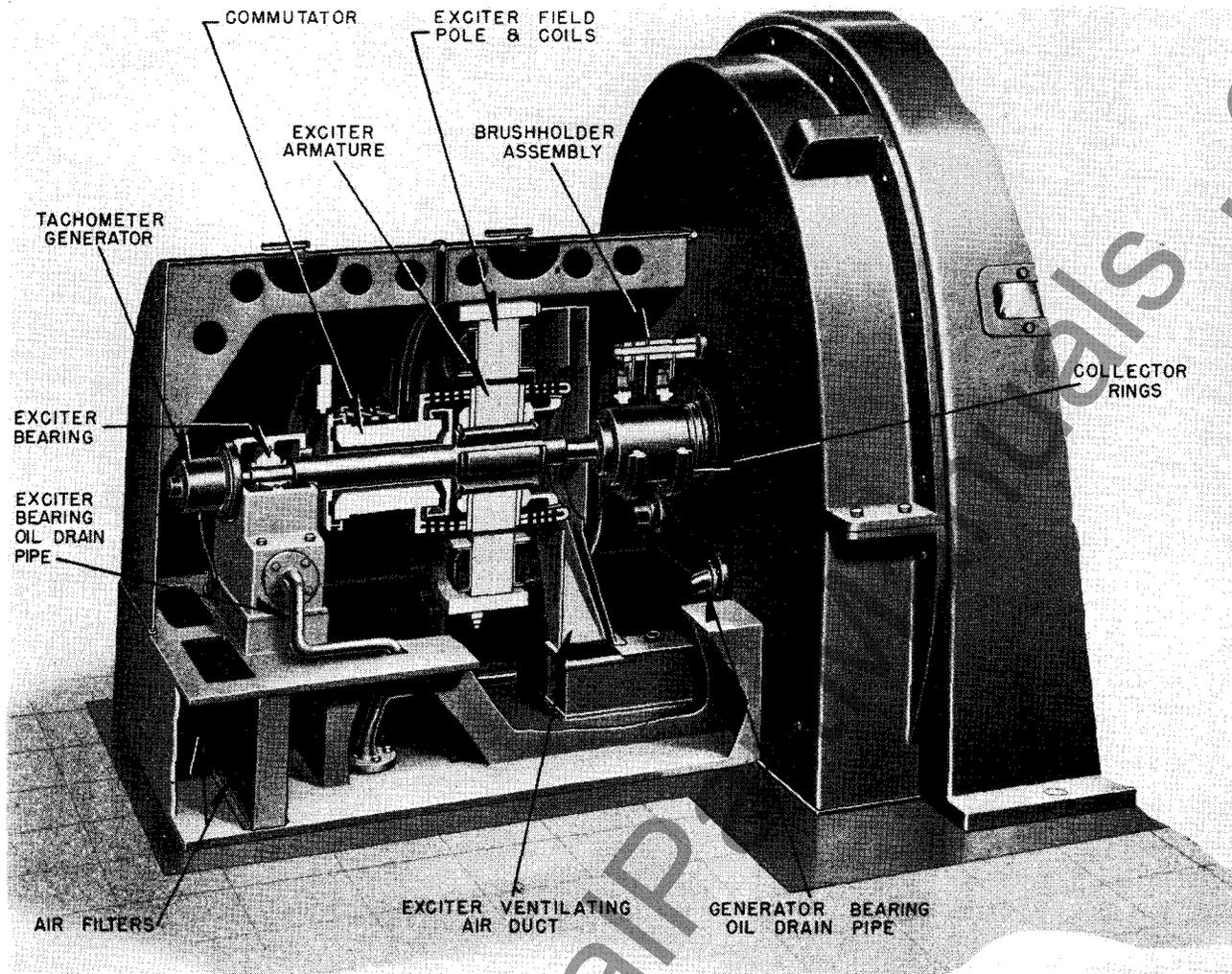
FIG. 11. Cutaway View of Exciter
