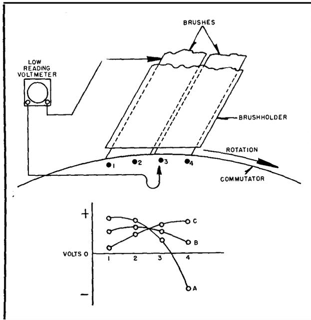
FIG. 28. Adjustment of Commutating-Pole Field Strength
