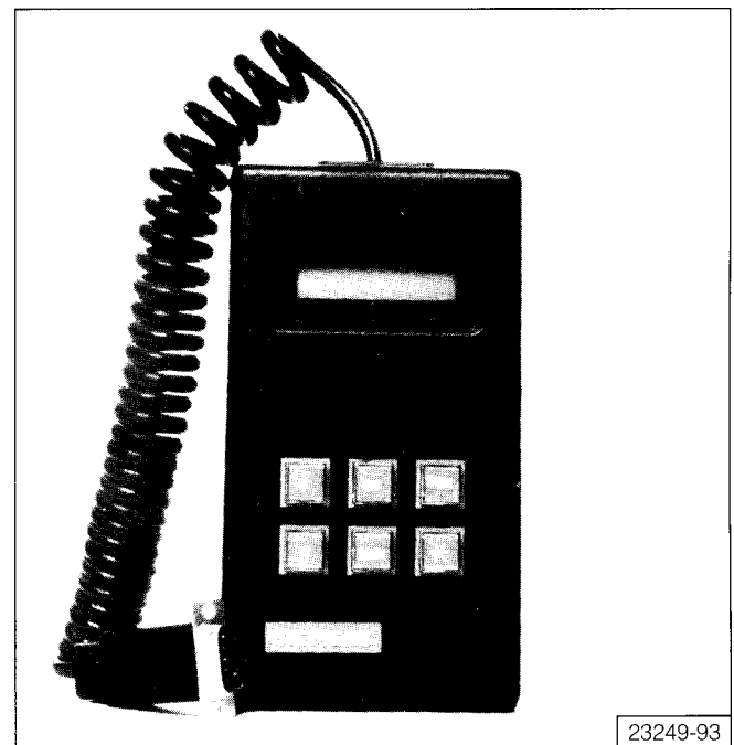
Figure 4: The SAMMS Hand Held Communicator.
