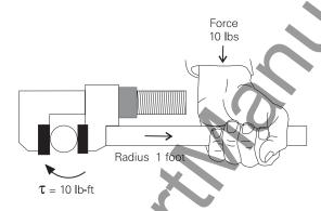
An increase in force or radius would result in a corresponding increase in torque. Increasing the radius to 2 feet, for example, results in 20 lb-ft of torque.
