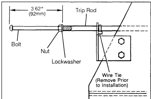
Figure 6. Latched Contactor
