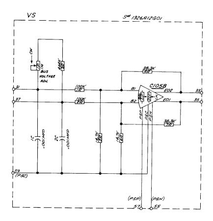
Voltage Sensor Schematic Diagram
