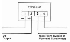
The Teleductor consists of a two-winding toroidal transformer having iron with specifically selected characteristics, a full-wave rectifier bridge, and loading and calibrating resistors. The two-winding transformer isolates the input circuit from the output circuit.
