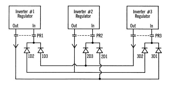
FIGURE 2 - VOLTAGE ERROR RESTRICTOR SCHEME
