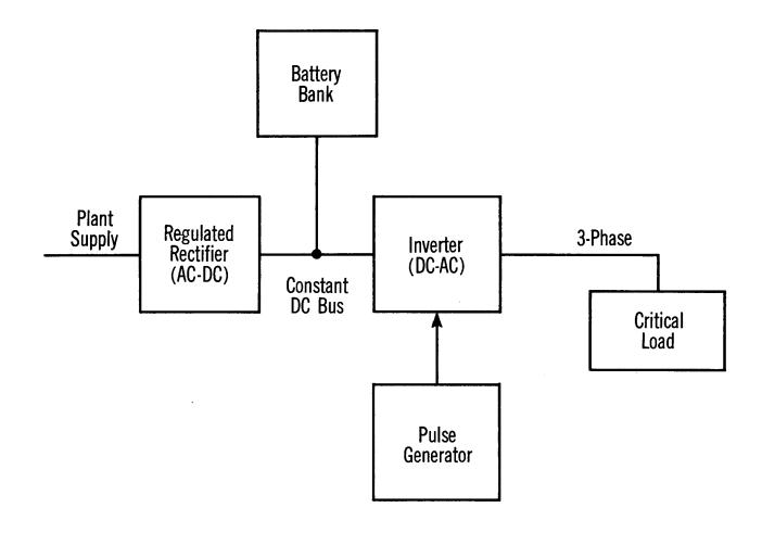
FIGURE 7 - BLOCK DIAGRAM OF FIXED FREQUENCY SINGLE INVERTER SYSTEM UNINTERRUPTIBLE POWER SUPPLY (UPS)
