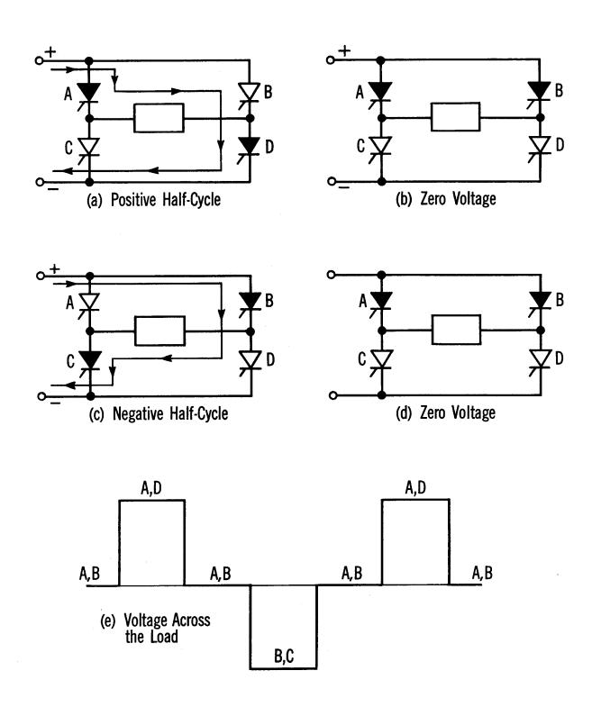
FIGURE 4 - SKETCHES SHOWING VOLTAGE CONTROL BY ADJUSTING PULSE WIDTH
