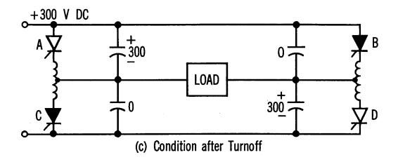
FIGURE 3 - SIMPLIFIED INVERTER BRIDGE SHOWING THYRISTOR TURNOFF ACTION
