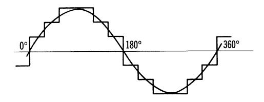
... with major harmonic components neutralized by the transformer connections, giving close to sine-wave operation.
