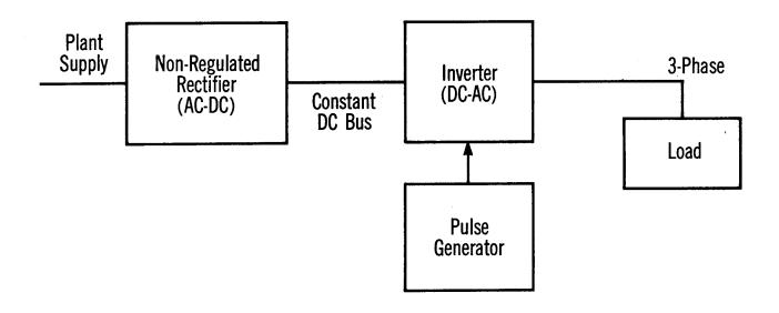
FIGURE 6 - BLOCK DIAGRAM OF STATIC FREQUENCY CHANGER OR POWER CONDITIONER (NO BATTERY REQUIRED)
