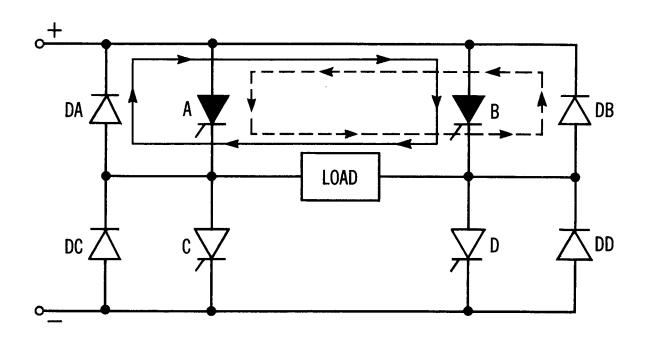
FIGURE 5 - SIMPLIFIED INVERTER BRIDGE SHOWING ADDITION OF FREE WHEELING DIODES TO ACCOMMODATE INDUCTIVE LOAD CURRENT
