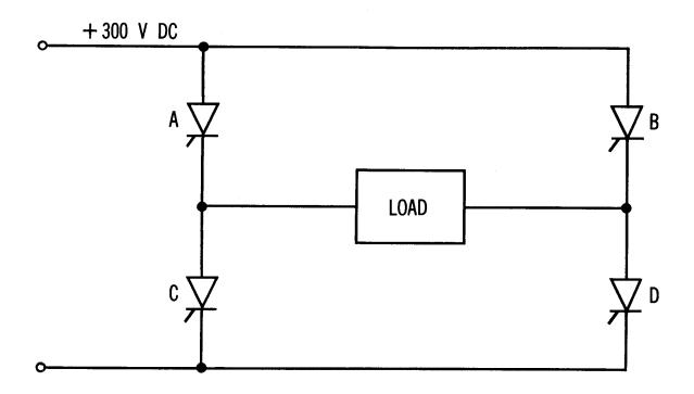
FIGURE 2 - SIMPLIFIED SCHEMATIC SHOWING REPLACEMENT OF CONTACTORS BY THYRISTORS
