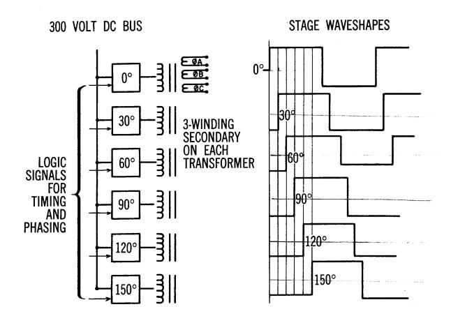
Wiring of transformer secondaries in patented harmonic neutralization scheme produces balanced three-phase output voltage. Minimum harmonic distortion results from cancellation effect.
