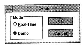
Real-time mode is the normal mode of operation for SIEServe software to collect data. Demo mode causes the devices of the present configuration to appear to be collecting and displaying real-time data.
