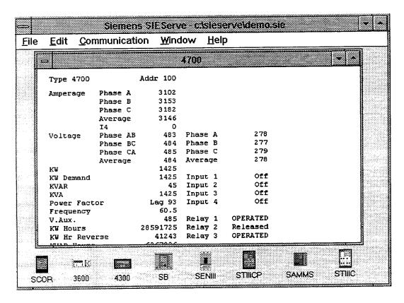
Notice that within the SIEServe application window are nine device icons, one for each type of ACCESS device supported by SIEServe software. Each time you minimize a device window, you will see the icon for that device type along with the device's unique name just below it. (Section 3.2 below talks about naming devices when you add them to your SIEServe system configuration.)
