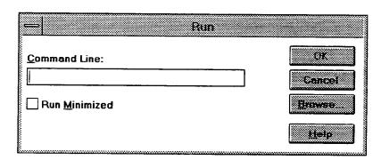
3. In the Command Line box, type the designation of the diskette drive where you've inserted the SIEServe diskette (either "a:" or "b:"), followed by "setup". Choose the OK button to complete the installation.
