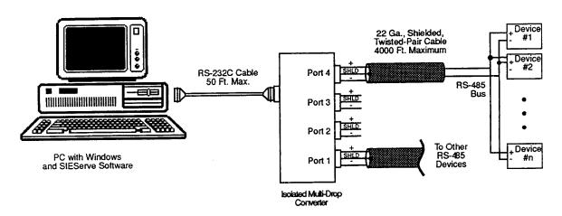
2. Use dial-up or short-haul modems and a Siemens Isolated Multi-Drop converter or a Power Measurements COM32 converter to connect a serial port on your computer to the SEAbus communications loop.
