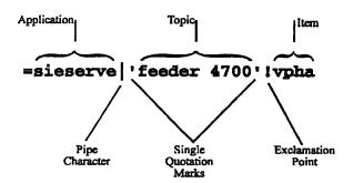
In this formula, "sieserve" is the *application* reference, "feeder 4700" is the unique name (or *topic*) of a particular device, and "vpha" is the *item* code for the data quantity, voltage on phase A. (The other characters are necessary components of the formula in Excel.) You can enter similar formulas in Excel (and other applications supporting DDE) for all data collected and displayed by SIEServe software. You can also request arrays of all real-time data for individual devices.
