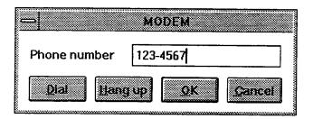
2. Enter the telephone number of the modem attached to your ACCESS system. (If you have special dialing requirements, such as the need to first connect to an outside line or to use a credit card, refer to Appendix C for information on modifying the dial string accordingly.) Choose the Dial button, and the Dial dialog box appears:
