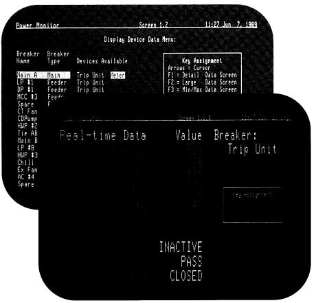
The "Detail Data Screen" (screen 1.2.1) for the "MCC#3" (Motor Control Center #3) circuit/trip unit reports: amps for each phase, ground amps and maximum phase amps as a percent of circuit breaker current sensor rating. It also reports which pickup is active, if any, the trip unit's self-test status and breaker position.
