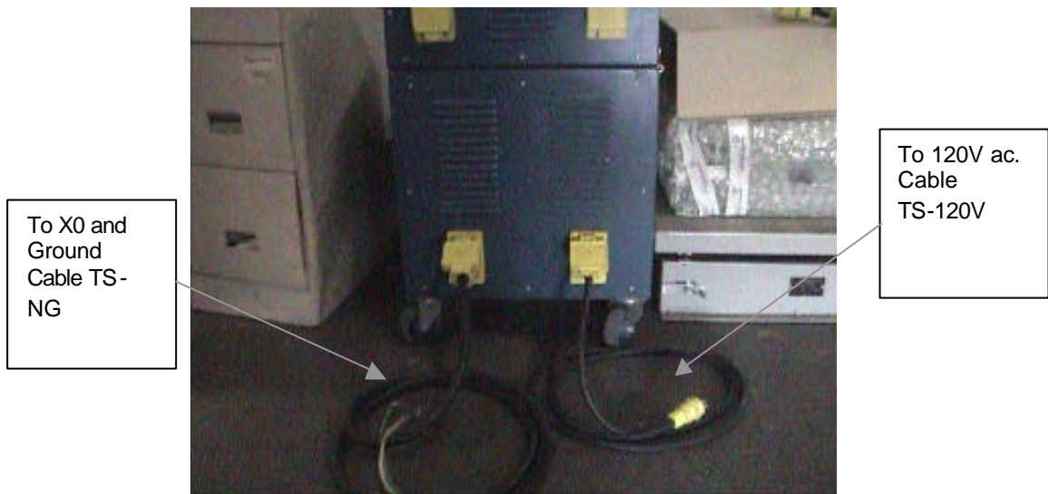
Figure 1. Connections for direct connection to system star-point
