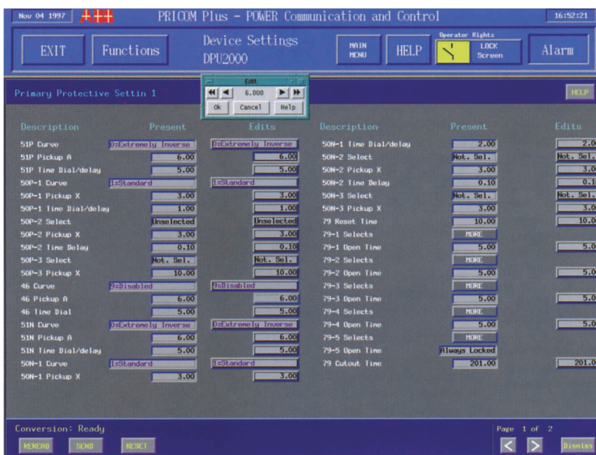
Selecting the Device Settings button provides the operator with this screen for review and editing the protective settings in the PRICOM-UE system.
