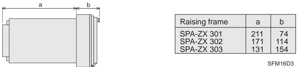
Fig. 3 Semi-flush mounting relay case (dimensions in mm)
