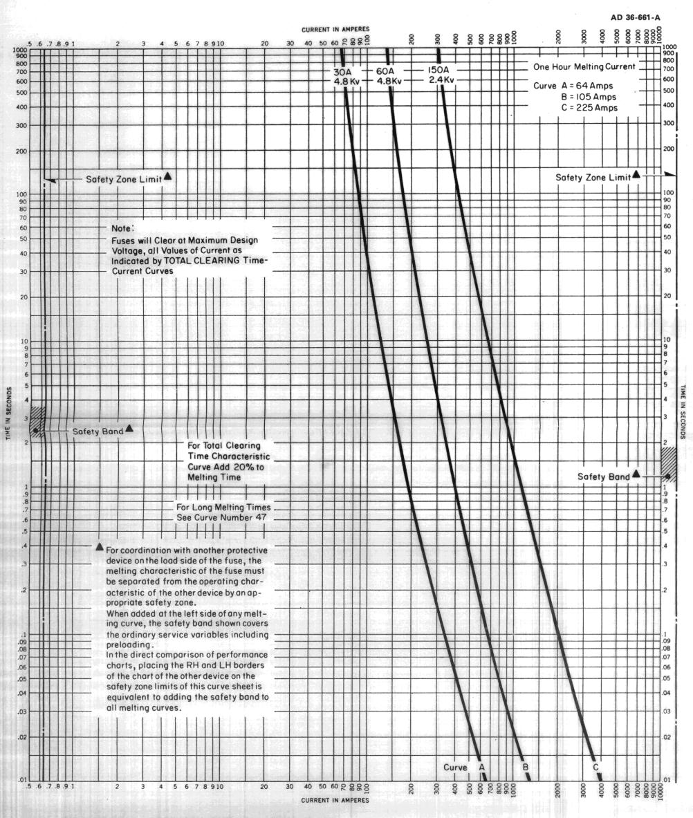
Type CLT-1 Current Limiting Power Fuses (EFD-1 Type)
