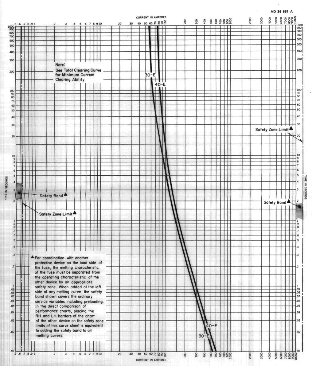
**Type CLE-1 Current Limiting Power Fuses** Melting time-current characteristics, 2.0 to 5.5 Kv
