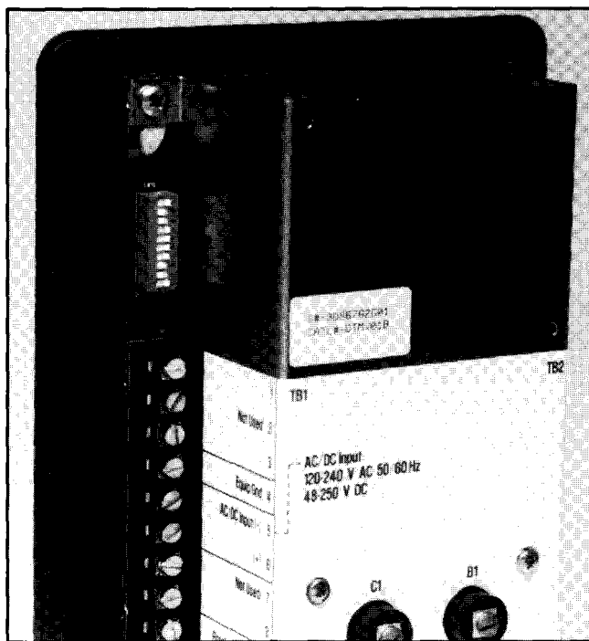
Figure 1-4 Digitrip MV Trip Unit With DIP Switches Shown in Upper Left (Rear View).
