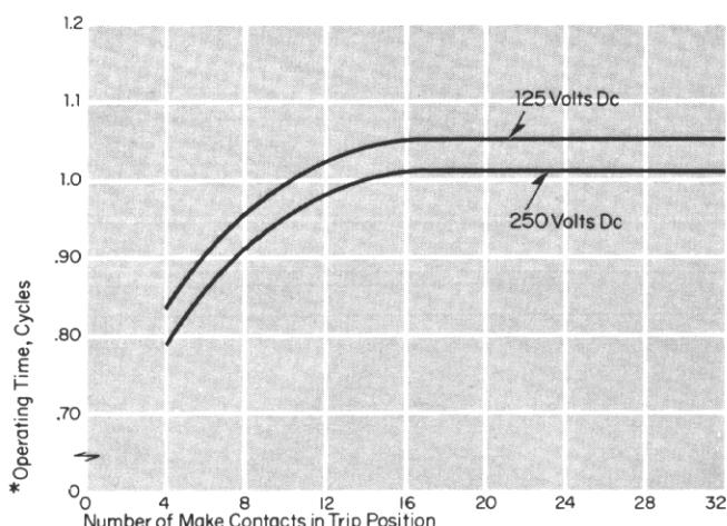
\*Operating Time is The Elapsed Time From The Initiation of The Pulsed Voltage to The Switch Coil till The Normally Open Contacts of The Switch Make
