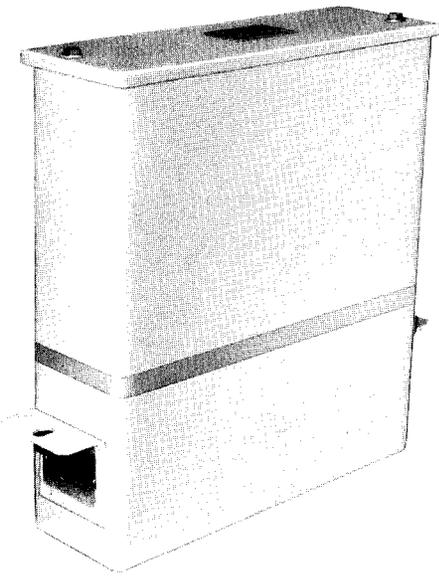
The replacement for PCB's (Inerteen®) in Westinghouse capacitors is a fluid called WEMCOL which is Isopropylbiphenyl (a synthetic aromatic hydrocarbon). Development of the new fluid began in 1970 and included detailed evaluations of more than 15 substances. WEMCOL was selected due to its excellent combination of environmental, electrical and flame resistant characteristics and because tests demonstrate clearly that capacitors with WEMCOL are very reliable and durable.
