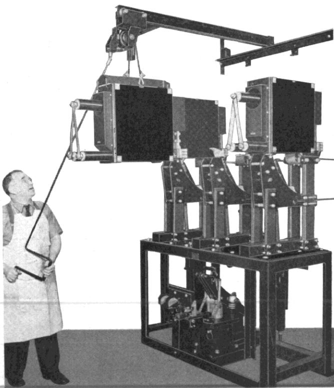
FIG. 3—USE OF STACK LIFTER WHEN INSTALLING OR REMOVING STACK OF TYPES 150-U-12 AND 150-U-22 "DE-ION" AIR CIRCUIT BREAKERS
