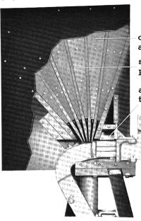
cooler assembly splitter plates arcing tip
