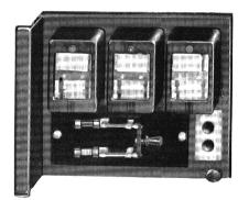
control panel is provided to make opening and closing operations on the breaker entirely automatic once the operator has moved the control switch either to close or trip the breaker. The control relays automatically govern the flow of compressed air to the mechanism and de-energize all magnet valve coils and relays after a closing or opening operation has been completed
