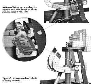
Both stationary and moving contacts are Cupaloy castings with silver-plated contact surfaces and with special arc-resisting metal inserts at points of arcing.
