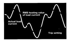
Siemens RMS sensing samples the entire current wave shape and calculates the effective heating value of the current. RMS sensing properly evaluates distortion on the line, provides accurate load protection and avoids unnecessary trips.
