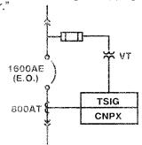
The above symbol is recommended for specifying the Static Trip III tripping system. The VT is only required for "CP" and "CPX" models
