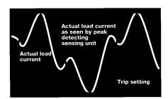
Harmonics distort the wave shape of current and can increase its peak value. Normal peak-sensing units are often confused and may trip, causing nuisance shutdowns, or may fail to trip, causing damage to the electrical plant.
