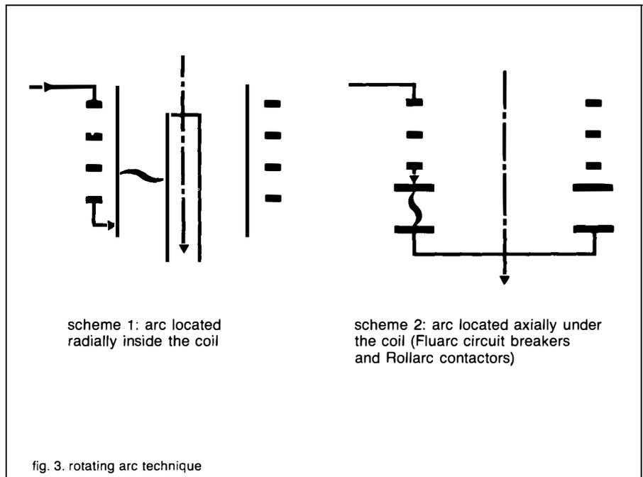
The speed of rotation of the arc has been measured. It varies with the intensity of the current to be interrupted and can reach the speed of sound in the gas for the highest currents.
