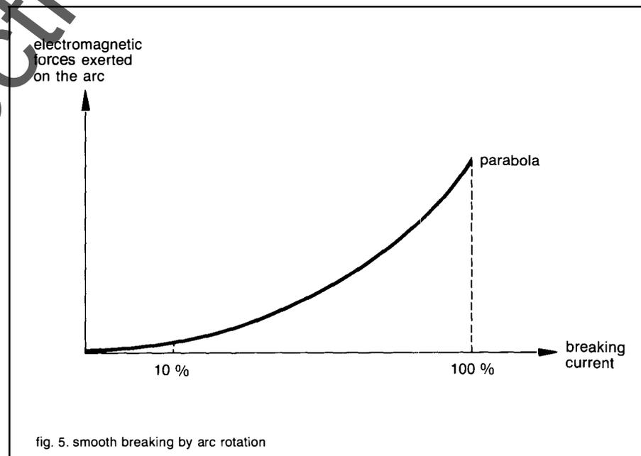
fig. 5. smooth breaking by arc rotation
