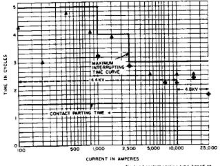
No load contact parting time based on 125/250V DC or 230V AC tripping
