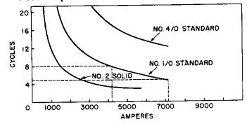
High-speed breaker reduces chance of line burn-down. Chart shows typical burn-down characteristics of covered copper wire at different interruption speeds.
