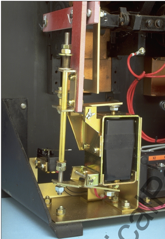
Fig. 25 Overview: Adjusting the Reset and Trip Assembly.
