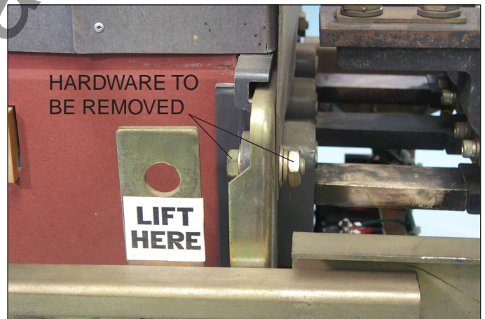
Fig. 10 Location of the Breaker Backplate Mounting Hardware.
