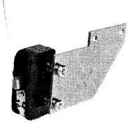
C. Making sure the Microswitch Spring Wire is behind the Interlock Bar, mount the Aux. Switch Assembly to the pre-drilled holes in the right Trip Unit Mounting Bracket, using the (2) .164-32 x .500" screws, (4) flat washers, (2) lock washers, and (2) nuts supplied.
