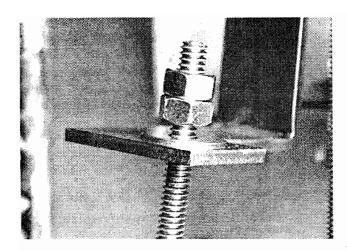
D. Align the holes in the DTA Assembly with the holes drilled in the right Breaker Side Plate in Step 3-B. Secure the DTA Assembly to the right Breaker Side Plate using the (2) .250-20 x .750" screws, (2) lock washers, and flat washers provided.
