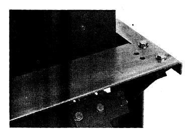
A. Using Drilling Plan A, drill and counter sink two (2) .375" holes in both the left and right Breaker Side Plates.
