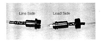
NOTE: The Load Side HV Wires are longer than necessary and are cut during the following steps. Before cutting the wires, be sure that sufficient length is left so that the connections can be made to the correct terminals on the CPT. Page 12 IL 33-DEH-1
