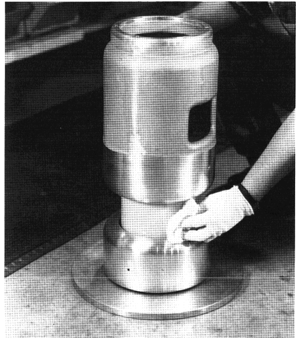
Plate 40: Placing the interrupter tube on the interrupter assembly fixture
