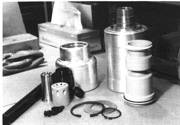
Plate 10: Components of the moving contact assembly
