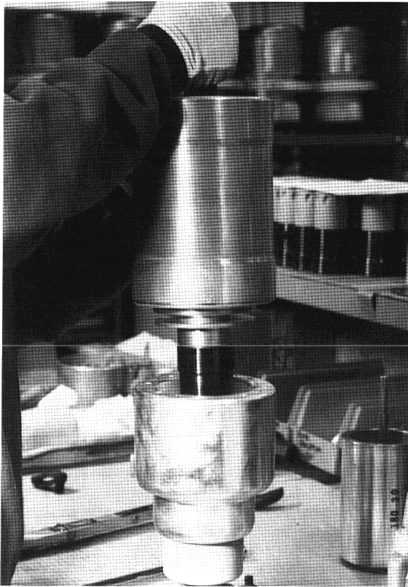
Plate 12: Retaining snap ring for the insulating nozzle
