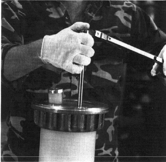
Plate 43: Re-installing the interrupter support tube
